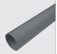
A rigid, halogen-free electrical installation conduit made of a special, grey (RAL 7037) plastic. The conduit is manufactured in straight 3 m bars. The conduit features a medium compression strength.
